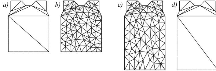
**Fig. 3.** When modifying the length of a T-shirt first the original underlying Delaunay triangulation gets changed (a, d). The coordinates of the refined triangles are then derived from their barycentric coordinates within this triangulation (b, c).
