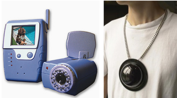
Fig. 2. (Left) ordinary wireless camera [10] and (right) wearable wireless webcam imitates surveillance cameras common in casinos and department stores [7].
