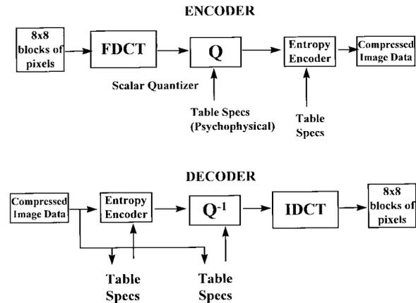
Fig. 2. Block diagram of JPEG encoder and decoder.
