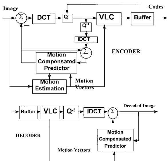
Fig. 6. Motion compensated codec for interframe coding.
