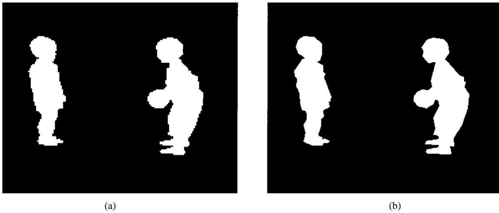
**Fig. 15.** Lossy encoding using a bitmap-based (a) and a contour-based (b) shape coder. The bitmap-based shape coder used pel replication as the upsampling filter (from [65]).
