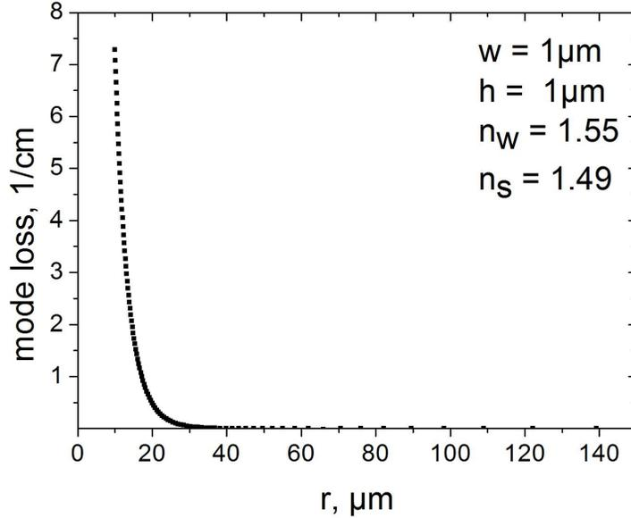
Figure 4: Simulation results: Bend losses of a circularly curved ridge waveguide with height  $h = 1 \mu\text{m}$  and width  $w = 1 \mu\text{m}$ .
