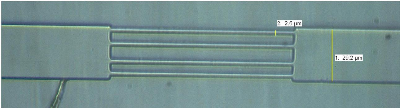
Figure 8. AWG fabricated with MPP.
