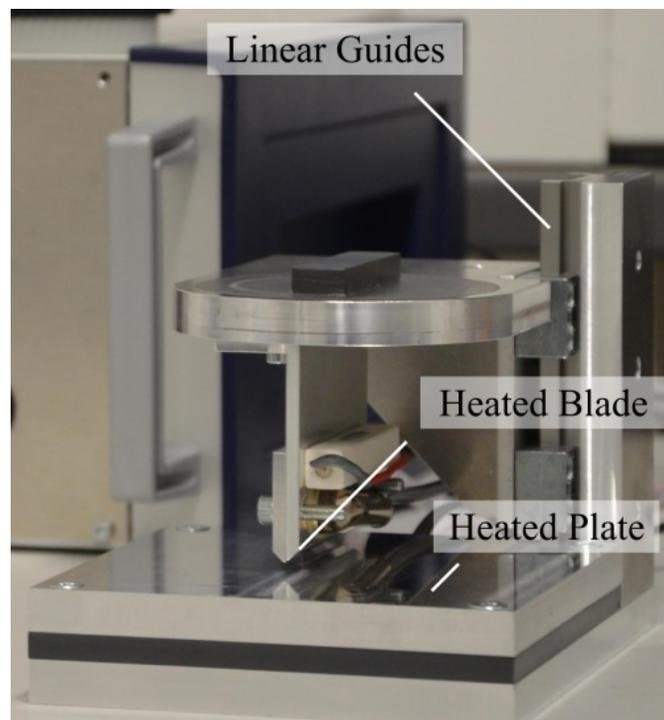
Figure 9. Photograph of the self made POF cleaver.
