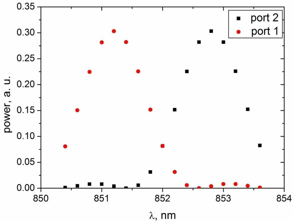
Figure 6. Simulated transmitted power as a function of wavelength for the two output ports.
