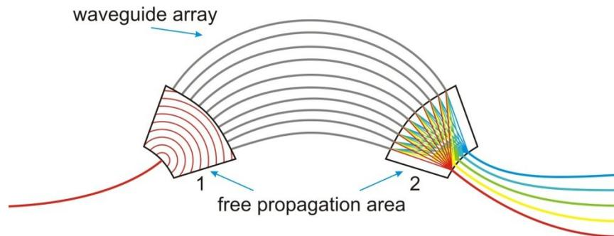
Figure 1. Schematic of an AWG.
