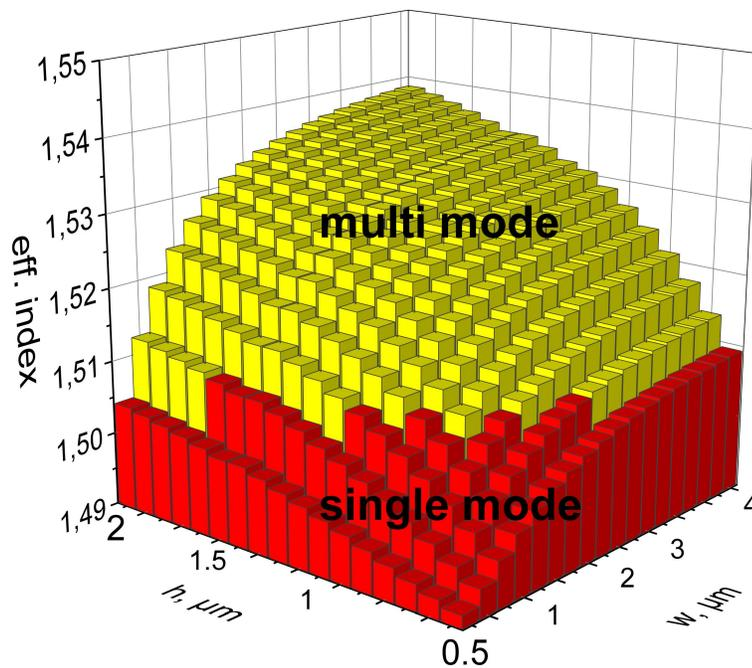
Figure 3. Results of the simulation for the waveguide calculated with FIMMWAVE Photon Design®.
