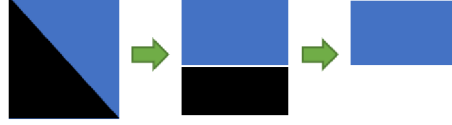
Figure 5: Using diagonal transformation, all of the redundant values in the lower triangle, depicted in black, are placed to the lower half of the matrix. Then, those rows can be removed.
