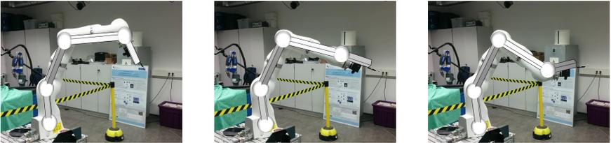
**Fig. 8.** Reconstruction of a sequence of an industrial robot moving along a path. The reconstruction is shown as an augmented overlay over the images.
