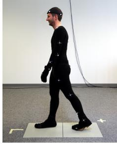
**Fig. 2.** A subject walking across the force plates in our laboratory setup
