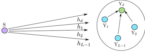
Fig. 1. System model, one source  $S$  and  $L$  receivers close to each other.  $S$  communicates a message to a destination node  $Y_d$ , all remaining receivers may serve as relays in order to assist  $Y_d$  in decoding the message. Independent channels  $h_d, h_1, \dots, h_{L-1}$  are assumed.
