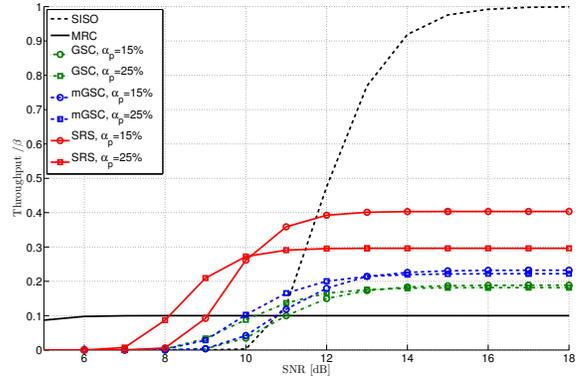
Fig. 5. Normalized throughput comparison between GSC, mGSC and SRS, with  $L = 4$  receivers,  $\alpha_p = \alpha/N_c = \{15, 25\}$  %, an OFDM symbol with  $N_c = 1024$  subcarriers with 16-QAM modulation, and bandwidth  $\beta$ .
