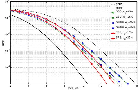
Fig. 2. The resulting BER comparison after cooperation. GSC, mGSC and SRS are considered with  $L = 2$  receivers,  $\alpha_p = \alpha/N_c = \{15, 25\}$  %, an OFDM symbol with  $N_c = 1024$  subcarriers with 16-QAM modulation.
