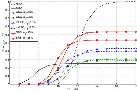
Fig. 4. Normalized throughput comparison between GSC, mGSC and SRS, with  $L = 2$  receivers,  $\alpha_p = \alpha/N_c = \{15, 25\}$  %, an OFDM symbol with  $N_c = 1024$  subcarriers with 16-QAM modulation, and bandwidth  $\beta$ .
