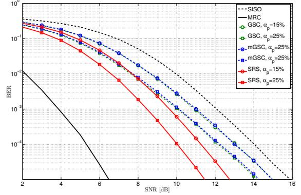
Fig. 3. The resulting BER comparison after cooperation. GSC, mGSC and SRS are considered with  $L = 4$  receivers,  $\alpha_p = \alpha/N_c = \{15, 25\}$  %, an OFDM symbol with  $N_c = 1024$  subcarriers with 16-QAM modulation.
