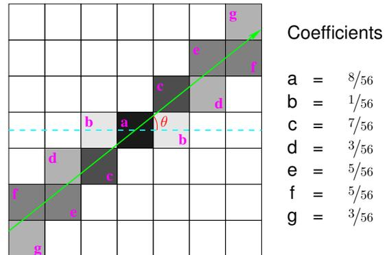
Fig. 1: Discrete version of linear motion blur ( $\theta = \arctan \frac{4}{5}$ )
