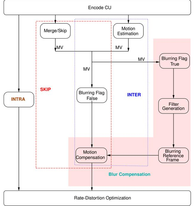
**Fig. 2:** Flow chart of motion blur compensation
