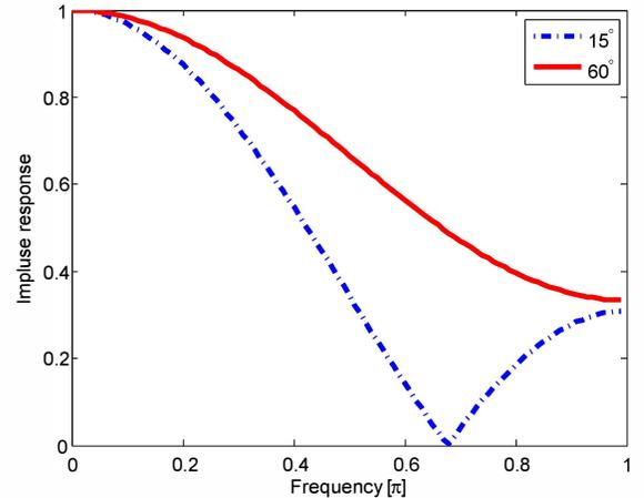
(b) Frequency responses alongside X-axis  $(\theta = 15^\circ, 60^\circ)$
