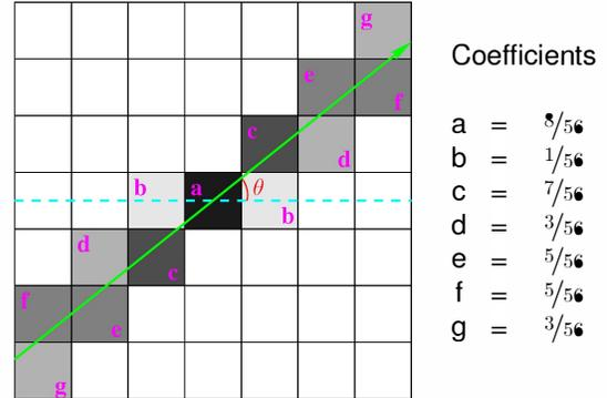
Fig. 1: Discrete version of linear motion blur ( $\theta = \arctan \frac{4}{3}$ )
