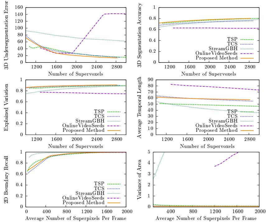
**Fig. 9.** Results generated for the dataset provided by [28] including scenes with diverse types of camera motion, motion blurring and non-rigid-motion. Please note the different abscissa. Higher values are better except for the 3D undersegmentation error and variance of area.
