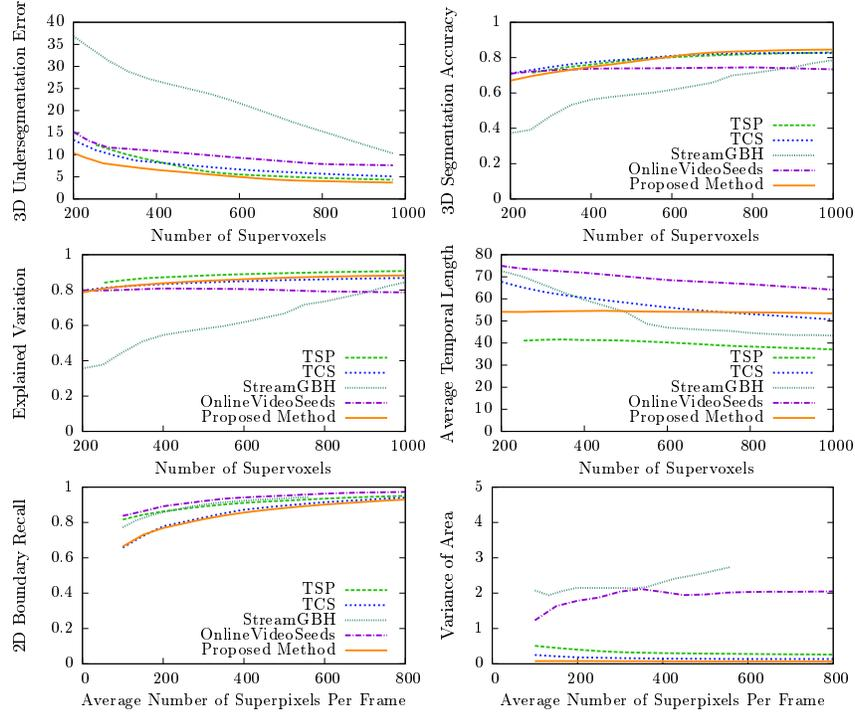
**Fig. 8.** Benchmark results for the dataset from [29] for state of the art supervoxel and superpixel algorithms for video content. Please note that the 2D boundary recall and the variance of area are plotted over the average number of superpixels per frame. Higher values are better except for the 3D undersegmentation error and variance of area.
