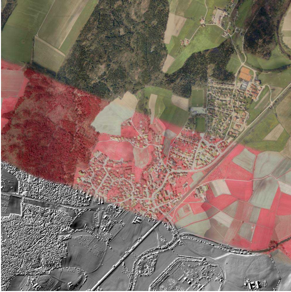
Figure 1: Multi-sensor Input Data (VIS, IR, Laser-scan) - TopoSys
