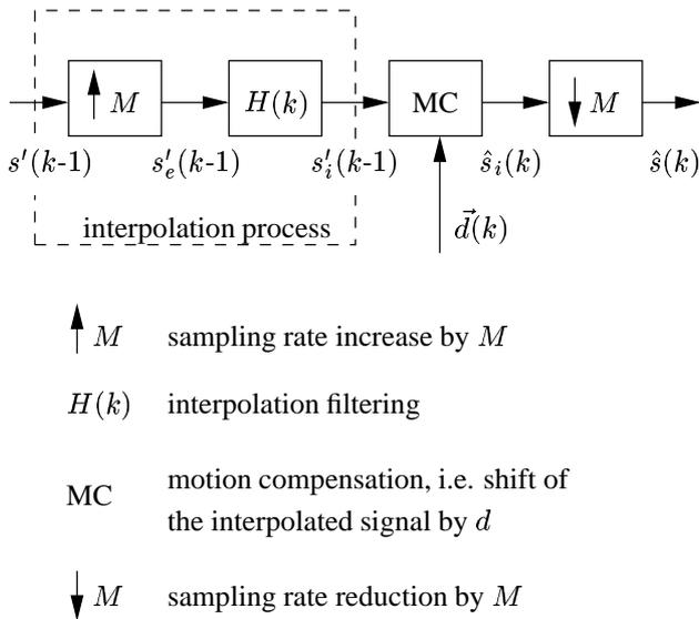
**Fig. 2.** Block diagram of the motion compensated prediction based on a displacement vector resolution of  $1/M$ .
