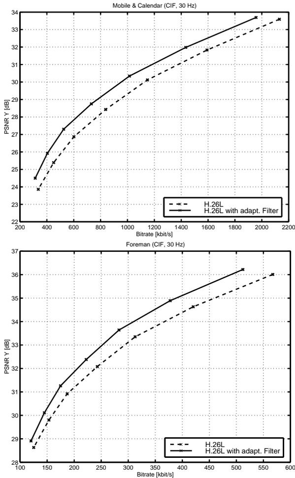
**Fig. 3.** Operational rate distortion curves for test sequences *Mobile & Calendar* and *Foreman*.
