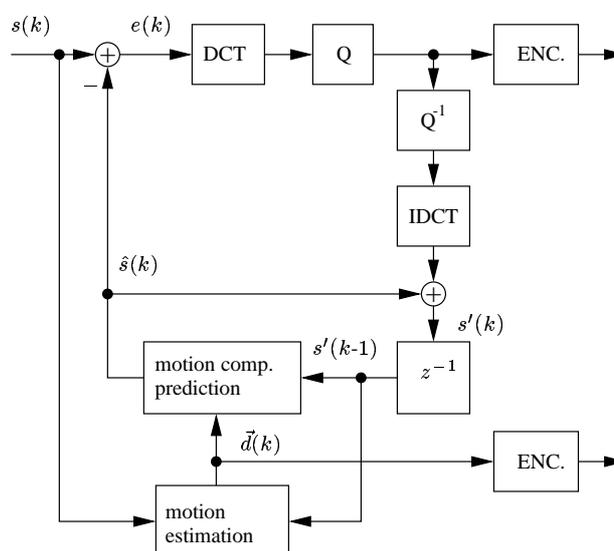
**Fig. 1.** Block diagram of a hybrid video encoder based on motion compensated prediction.
