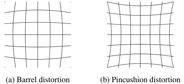
Fig. 3. Possible types of radial distortions.
