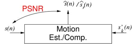
**Fig. 6.** Comparison between input signal  $s(n)$  and motion compensated output once with and second without in-loop radial distortion compensation.
