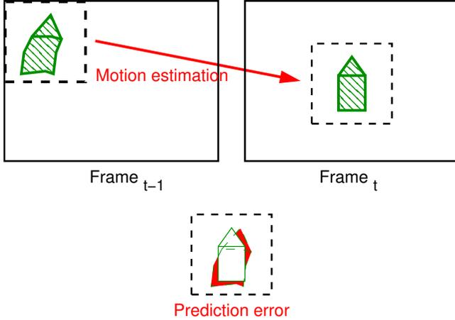
**Fig. 5.** Principle where the coding gain due to radial distortion compensation in hybrid video coding comes from: the house is different distorted due to radial lens distortion in frames  $t$  and  $(t - 1)$ . The resulting systematical prediction error within the motion estimation is depicted in the lower picture.
