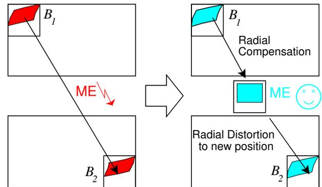
**Fig. 1.** Principle of radial distortion compensation in motion compensating video coding: the real object in block  $B_1$  moves translational resulting in different image blocks  $B_1$  and  $B_2$ . In an in-loop radial distortion compensating system (Figure right) the matching process works better since the shape distortion was adjusted to match the new position.
