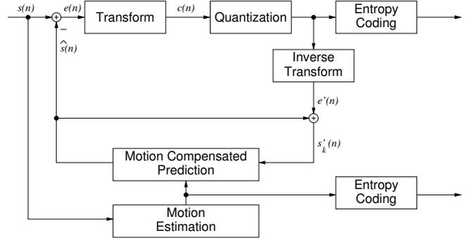
Fig. 2. Simplified block diagram of a hybrid video coder.
