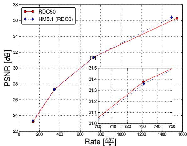
**Fig. 8.** RD diagram for test sequence *Flower Garden* (CIF) with  $k_c = 50$ . The solid line corresponds to the proposed algorithm, the dash-dotted line is the HM-5.1 reference.
