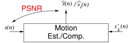
**Fig. 6.** Comparison between input signal  $s(n)$  and motion compensated output once with and second without in-loop radial distortion compensation.
