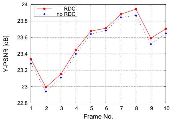
**Fig. 7.** Frame-wise evaluation of the output of the motion compensated prediction signal.
